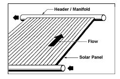
Solar collectors are made of a variety of materials. Collectors that operate only when temperatures are above freezing can be made of lower cost materials such as thermoplastic rubber or polypropylene. These collectors can be used in the far southern part of the U.S. and for all outdoor seasonal use pools in the rest of the U.S.
