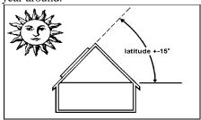
For summer only heating, use latitude minus 10-15°. For winter only heating, use latitude plus 10-15°. For year around heating, install the collectors at latitude. Variations from these ideals can be compensated for by adding additional collector area.
